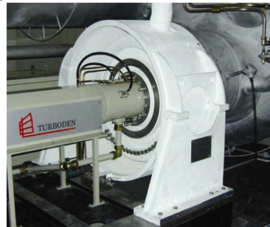
Two-stage axial turbine for the biomass-fired ORC process
